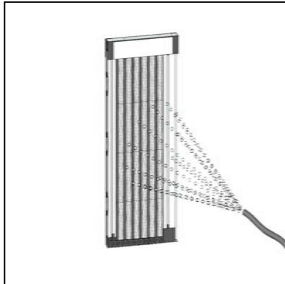
To clean the gauze, lean it against a wall. Spray the gauze with water and clean it using a brush. Be careful not to damage the folds in the gauze when doing this.
