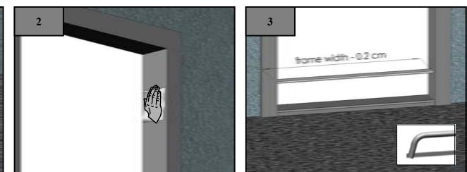
The doorframe and threshold must be dry and free of dust and grease.
