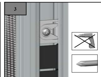
Loosen the screw mounted on the small white plate several turns.
