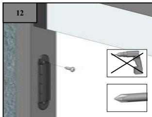
Remove the protective layer from the strips. Slide the mounting side against the doorframe to determine the position of the mounting clips.
