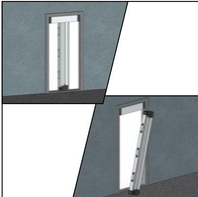
Open the door and pull the mounting frame firmly from the mounting clips. The door can be easily removed by pulling the gauze bundle at a slight angle.
