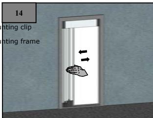
Press the mounting frame firmly against the mounting clips.
