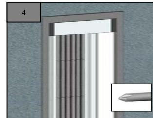
Adjust the pull strip vertically and retighten the screw. Press the cover plate back into place.
