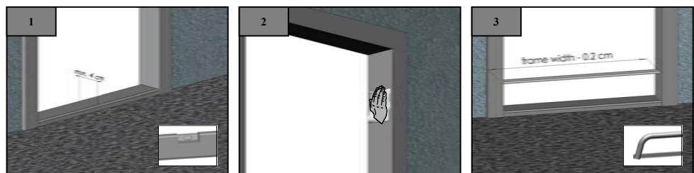
The concertina screen door must be mounted on a level threshold (minimum width 4 cm).
