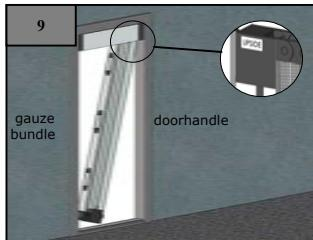
Mount the lower rail on the threshold directly under the upper rail. Remove the protective strip. Press firmly.
